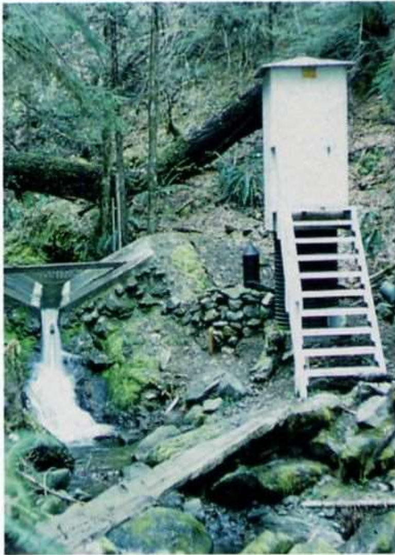
Gaging station to monitor streamflow on a small watershed, H. J. Andrews Experimental Forest, Willamette National Forest, Oregon.
