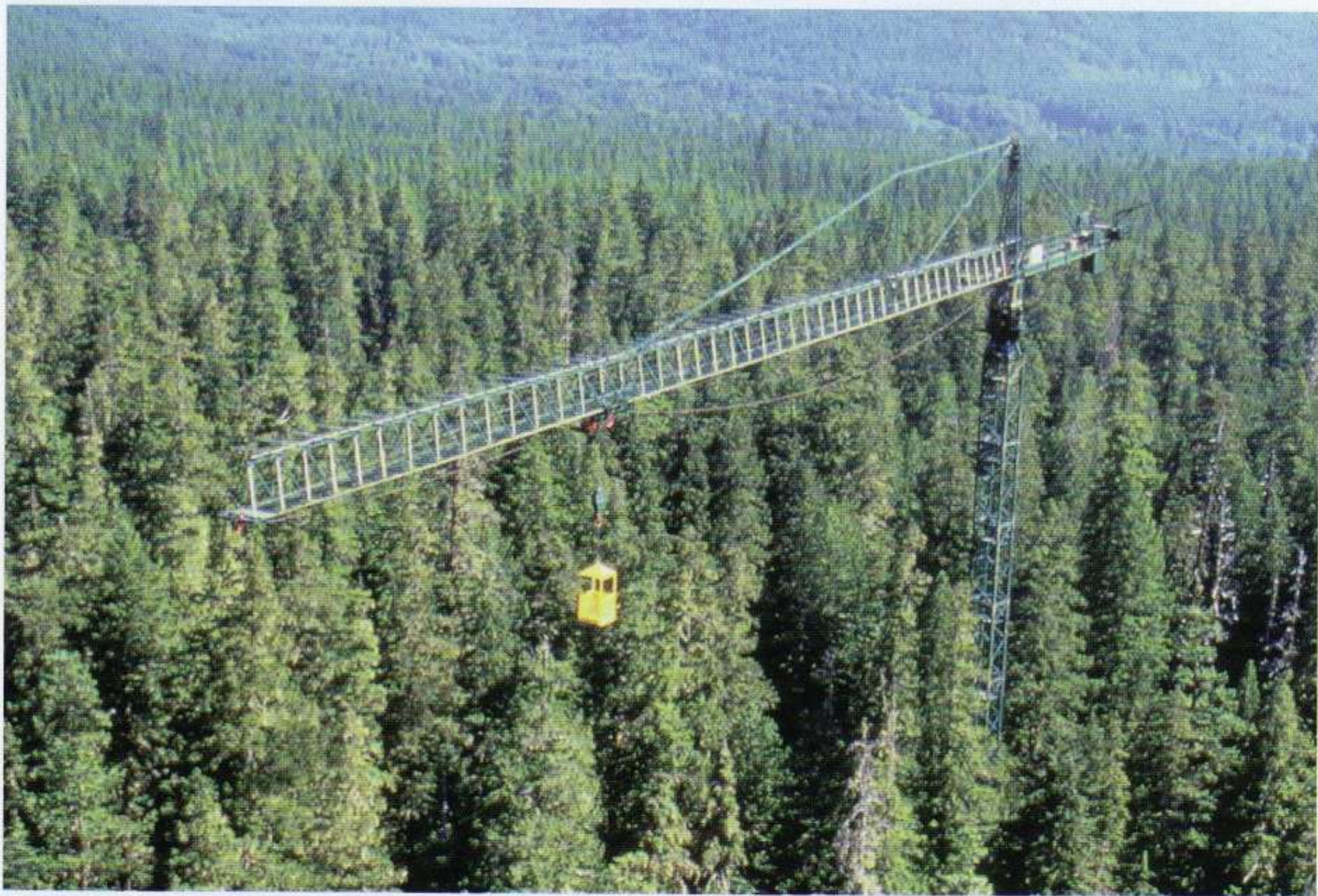
Construction crane providing access to 5.6 acres of old-growth Douglas-fir–western hemlock forest at Wind River Canopy Crane Facility, Gifford Pinchot National Forest, Washington.
