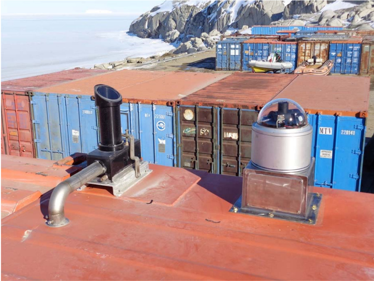
Figure 4 – on the left the VELOD (Vertical looking Device - operational since February 2013) and on the right the alt azimuth platform called MIGE (Multiple Input Geometry Equipment - setup in November 2014). Both systems are connected to the spectrometer via fiber optics.
