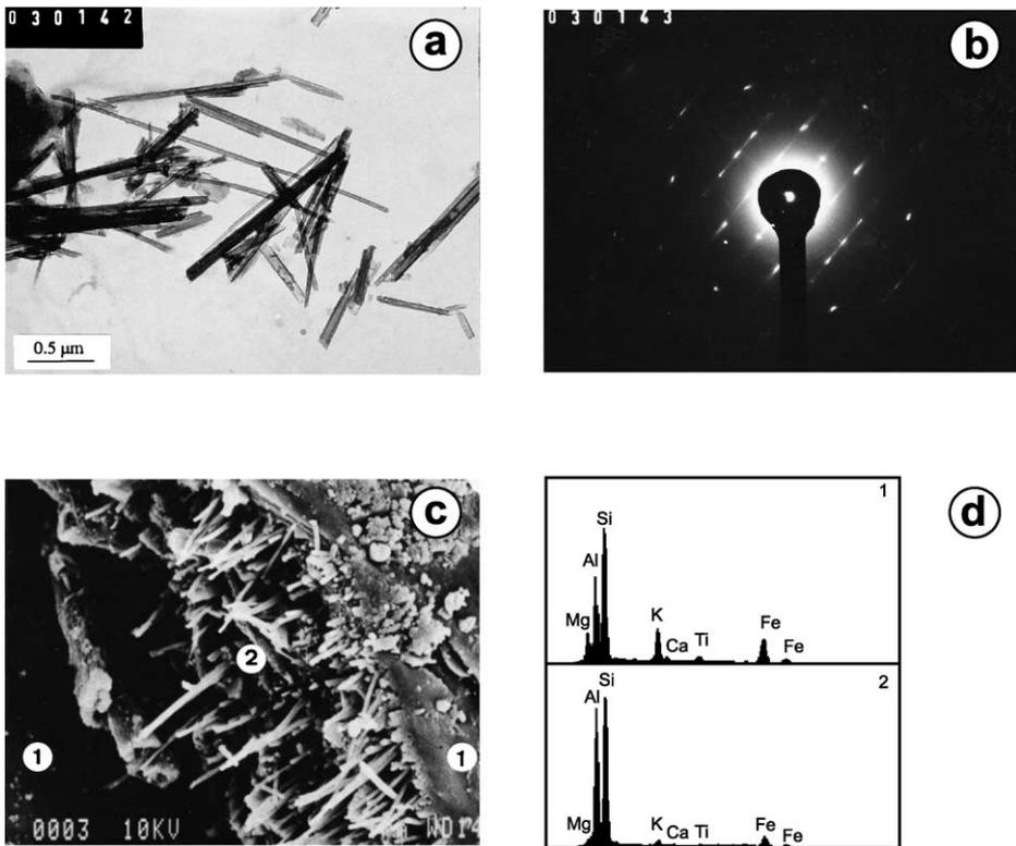
Fig. 5. TEM images: (a) double tubes of metahalloysite, (b) X-ray microdiffraction diagram within a tube from image (a). SEM-EDS images, (c) weathered biotite from granitic saprolite, (d) chemical spectrum of biotite-position 1 and kaolinite–metahalloysite-position 2.
