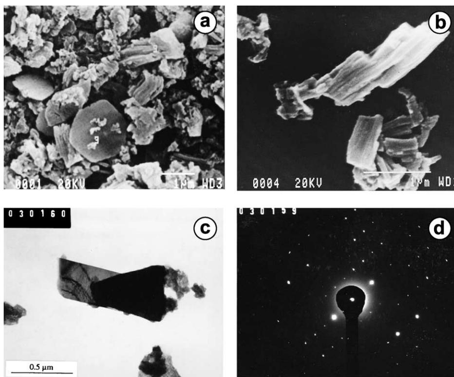
Fig. 6. Micromorphology of gibbsite in granitic saprolites from Cávado river basin, SEM-EDS images: (a) hexagonal plates and (b) prisms or lathes. TEM images: (c) wedge like particle and (d) X-ray microdiffraction diagram of gibbsite.
