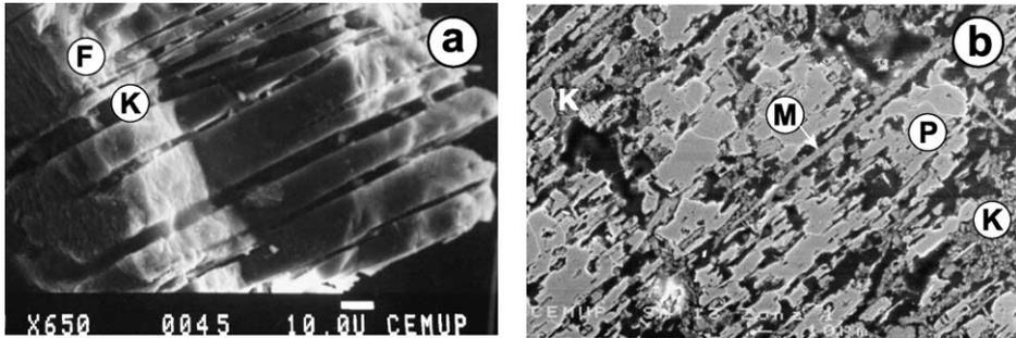
Fig. 7. SEM-EDS images of granitic saprolites: (a) weathered feldspar (microcline) from Cávado river basin, showing kaolinite plasma between the cleavage surfaces; (b) etch-pits on plagioclase from Oporto granite and kaolinite in its weathering microsites. F = feldspar; P = plagioclase; M = muscovite; K = kaolinite.
