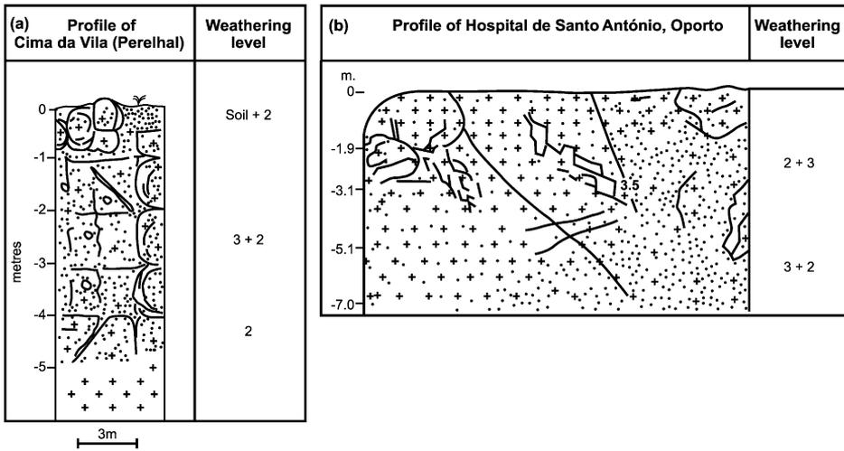
Fig. 2. Sketch of weathering profiles; (a) Cávado river basin—Perelhal granite—Cima da Vila profile; (b) Oporto granite—Hospital de Santo António profile. 2 = Weathered rock; 3 = granitic saprolite.
